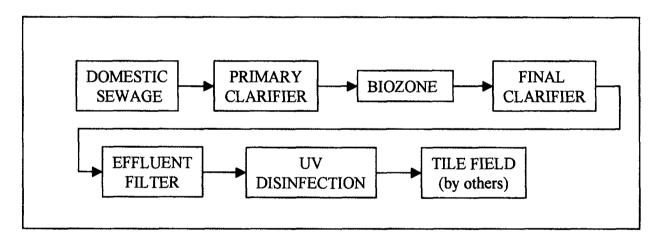
The Klargester HQ treatment plants are the latest innovation in the development of our package sewage treatment plants. Guaranteed to produce an effluent quality of  $\leq 10$  mg/l BOD<sub>5</sub>,  $\leq 10$  mg/l Suspended Solids and  $\leq 400$  MPN/100ml fecal coliform, the HQ series meets the requirements of the current Ministry of Health's Innovative Technologies Program.
